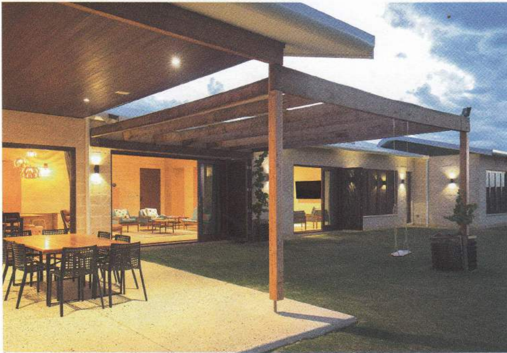
④ A northern outdoor dining area with a solid roof was required to block the northerly sun from the internal dining room to improve the overall building performance – this approach would not be appropriate in cooler climates.
