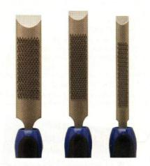
Available in a set of three - 13mm, 19mm and 25mm — these tools are suited to a variety of wood-shaping tasks.
