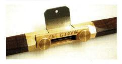
This shave is 235mm long x 12mm wide x 12mm high. It weighs 90g and is fitted with a 19mm wide x 1.2mm thick x 24mm long tool steel or HSS blade. It has a 60° blade angle for planing. The all-brass sole has a radius of 9.5mm ( $^{3}/_{8}$ ").
