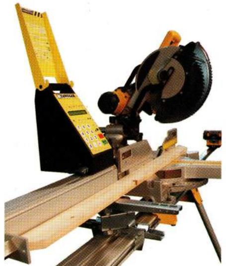
Simply enter a dimension on the keypad and the SawGear will adjust the end stop as required. Place your material against the stop and make your cut, straight or mitre. The SawGear accessory is easy to use, accurate, portable and ruggedly made to stand up to adverse site conditions.
