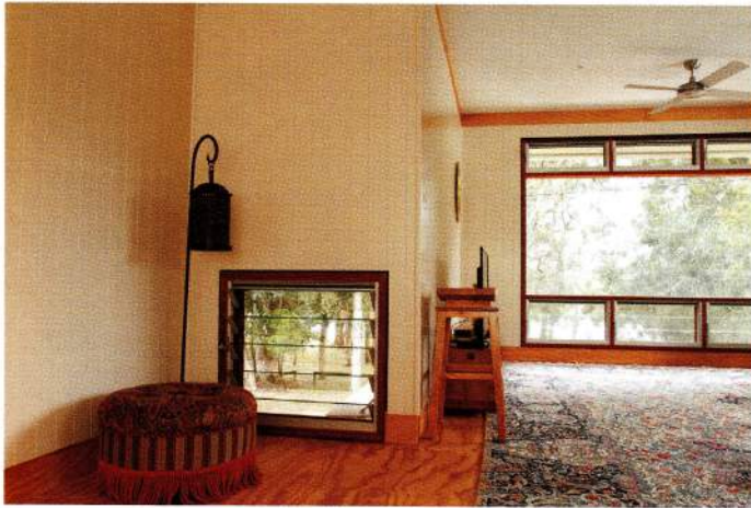
Homeowner Karen uses this light northeast-facing rumpus room to run yoga classes. FSC plywood lines the floor and louvre windows vent hot air from the space.
