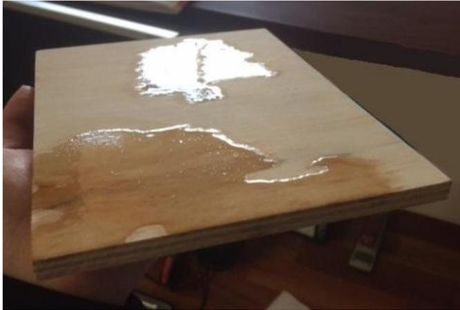
Here we applied 2 coats of the countertop oil. For testing purposes and to ensure as much penetration as possible, it was applied heavily and we did not remove the excess oil off the surface. It was also allowed to dribble over the edges to assess the cross cut.
