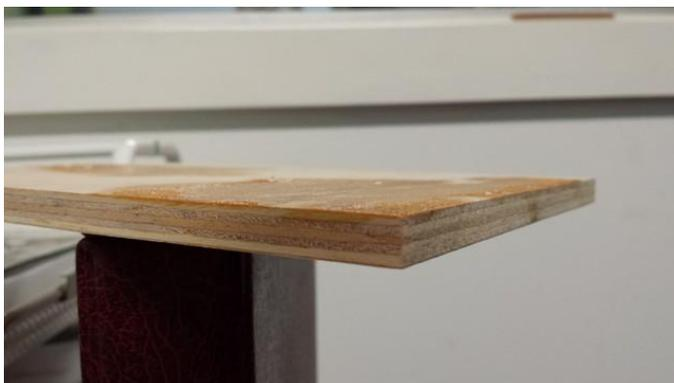
Three weeks later, there is absolutely no cupping, separation or delamination of the surface.
