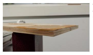
Three weeks later, there is absolutely no cupping, separation or delamination of the surface.
