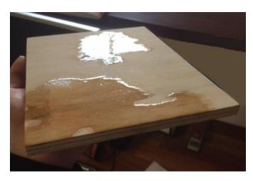
Here we applied 2 coats of the countertop oil. For testing purposes and to ensure as much penetration as possible, it was applied heavily and we did not remove the excess oil off the surface. It was also allowed to dribble over the edges to assess the cross cut.
