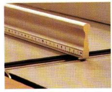
The straight edge is just under 47mm high with a comfortable-to-use hourglass shape. It is stable enough to stand upright on its own, leaving the user with both hands free for other tasks.
