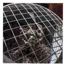
L—R: The hemp as supplied; a special mortar mixer was required to cope with the sticky hemp mixture; a range of shapes and sizes for the tampers enabled all areas to be reached.
