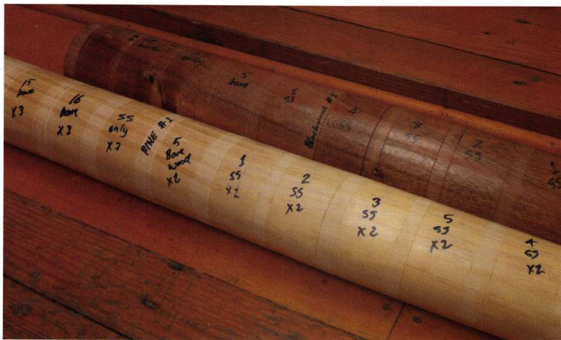
Left: 100mm dia sections of radiata pine and blackwood were trued and sanded. Test strips were separated with turned 'gaps' which showed a bare wood contrast. Each section showed the number that denoted a certain product.
